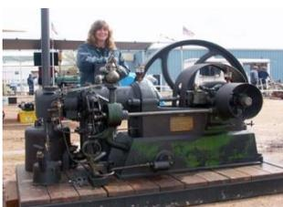
Figure 1: Hornsby-Akroyd vapourising oil engine: Richardhornsbyvaporizing oilengine.jpg
